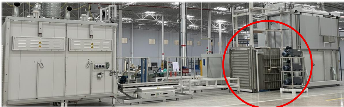
Example CAB line: with Dryer/Preheater and Vacuum Lock and Tower Furnace
