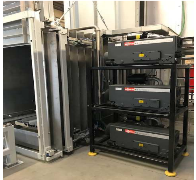
increased speed by Triplex vacuum pump to reduce cycle time
