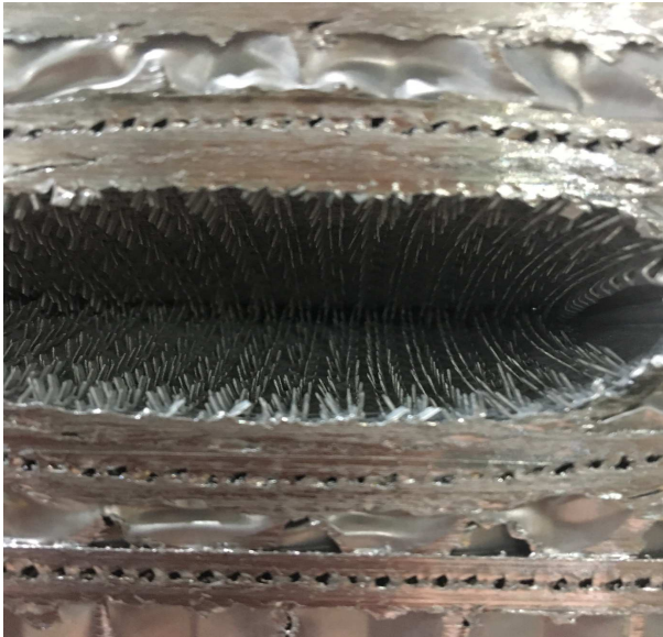
Excellent results on brazing of inner fins at burst / pressure test
